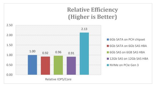
The second major benefit is NVMe/PCIe uses less than half the number of CPU instructions to process an I/O request when compared to SAS or SATA.
