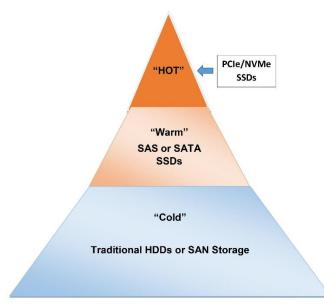
As an example, the following storage configuration would accelerate performance over a solution entirely based upon HDDs.
